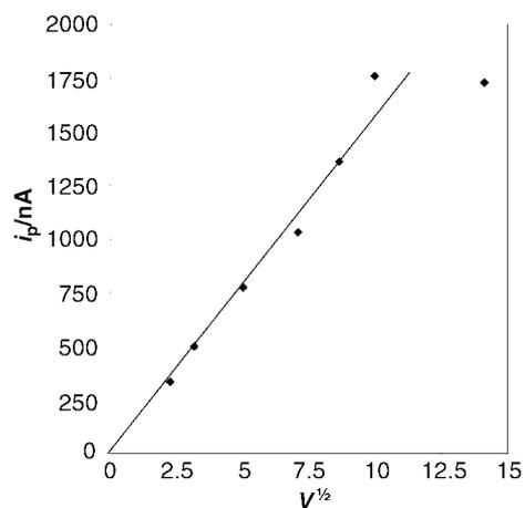
Fig. 3 Plot of  $i_p$  versus  $v^{1/2}$  for cyclic voltammograms of  $2 \times 10^{-5} \text{ M}$  1-naphthol in 0.5 M phosphate buffer, pH 6.65 for scan rates ( $v$ ) from 5 to  $200 \text{ mV s}^{-1}$ .  $E_i = 0 \text{ V}$ ;  $E_{\text{sw}} = +1000 \text{ mV}$ .
