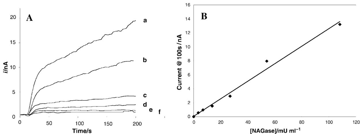
**Fig. 8** Electrochemical assay of NAGase in buffer solution. (A) Amperograms obtained for NAGase at: (a) 108; (b) 54; (c) 27; (d) 13.6; (e) 6.8 and; (f) 3.1 mU ml<sup>-1</sup> final concentration. (B) Calibration plot.
