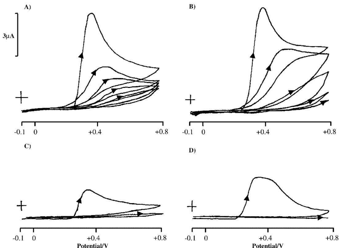
Fig. 2 Cyclic voltammograms of  $2 \times 10^{-4} \text{ M}$  1-naphthol in 0.5 M phosphate buffer, pH 6.65 at a SPCE under quiescent (A, C) or hydrodynamic (B, D) conditions, showing five repeat cycles at  $50 \text{ mV s}^{-1}$  (A, B) or two repeat cycles at  $5 \text{ mV s}^{-1}$  (C, D).
