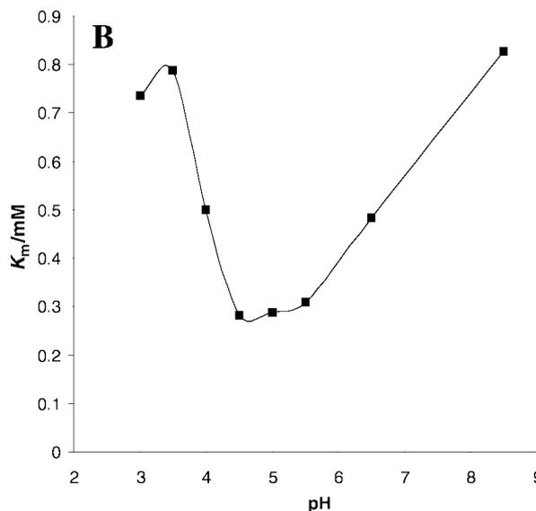
**Fig. 6** Plots of (A)  $V_{\text{max}}$  and (B)  $K_m$  versus pH for NAGase measured amperometrically at SPCEs in stirred phosphate buffer containing 1-naphthyl-*N*-acetyl- $\beta$ -D-glucosaminide as substrate.
