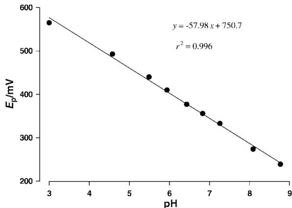
**Fig. 4** Plot of  $E_p$  versus pH obtained from cyclic voltammograms of  $2 \times 10^{-4} \text{ M}$  1-naphthol in 0.5 M phosphate buffer.  $E_i = -100 \text{ mV}$ ;  $E_{\text{sw}} = +800 \text{ mV}$ .
