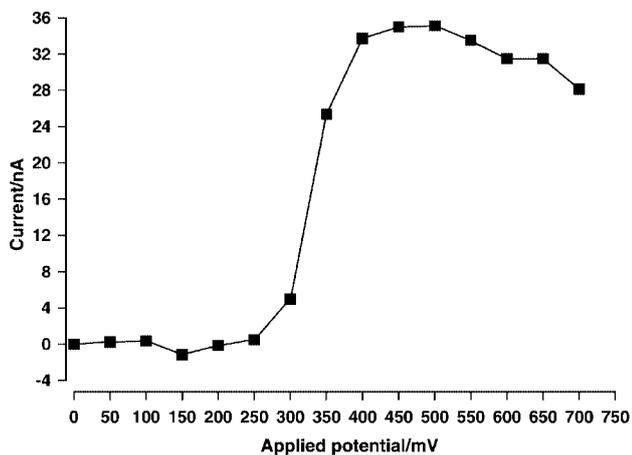
**Fig. 5** Hydrodynamic voltammogram for a solution of  $4 \times 10^{-6} \text{ M}$  1-naphthol in 0.5 M phosphate buffer.
