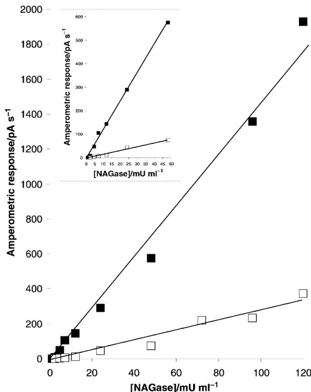
**Fig. 7** Calibration plots obtained under hydrodynamic conditions for NAGase added to phosphate buffer solution containing 3.75 mM 1-naphthyl-*N*-acetyl- $\beta$ -D-glucosaminide substrate at pH 4.5 (solid squares) or pH 6.5 (open squares). Inset shows expanded lower concentration range for clarity.
