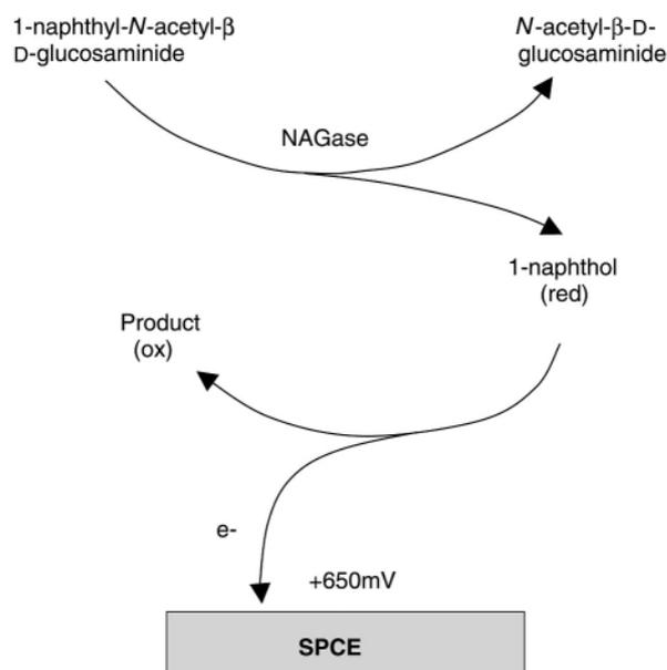
Fig. 1 Schematic diagram for the electrochemical assay of NAGase.
