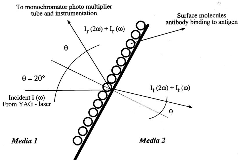
Fig. 1. Second harmonic generation from an interface between media.  $I_r(\omega)$  and  $I_t(\omega)$  are reflected and refracted fundamental beam, respectively.  $I_r(2\omega)$  and  $I_t(2\omega)$  are surface second harmonic signals generated by  $I_r(\omega)$  and  $I_t(\omega)$ .
