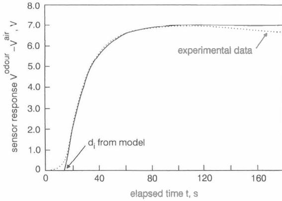
**Fig. 3** Graph showing effect of fitting four-parameter second-order model to actual sensor response
