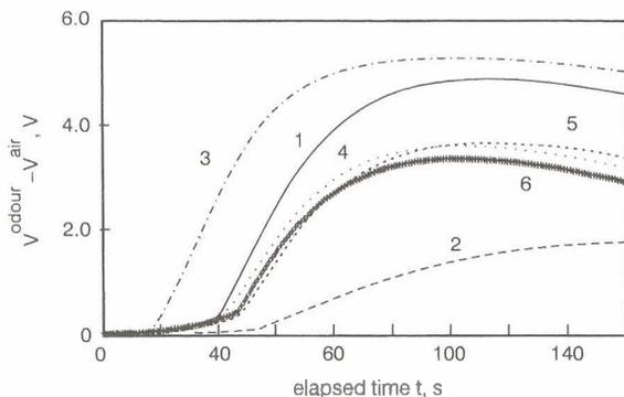
**Fig. 2.** Typical dynamic response of array of six odour sensors to pulse of odour delivered by sampling device, i.e. the breath of a cow. Signal voltage  $V$  is proportional to sensor resistance. The number by each curve refers to sensors listed in Table 1
