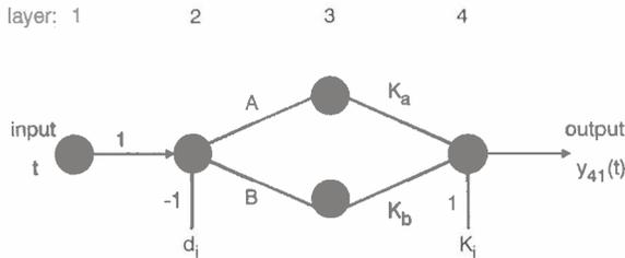
**Fig. 4** Neural network used to estimate values of four sensor parameters in our second-order model
