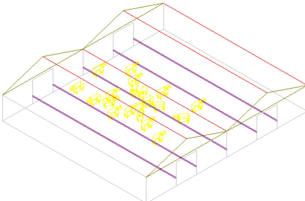
*Figure 4. Wireframe rendering of the simulation setup in RPS for modelling an entire byre complete with a small herd of 20 cows. The byre is 36 m long, 36 m wide and 8 m high at the highest point. The cows are shown in yellow. The fences are shown in purple. The roof is shown in red and the gables in green. The floor and walls are shown in grey.*
