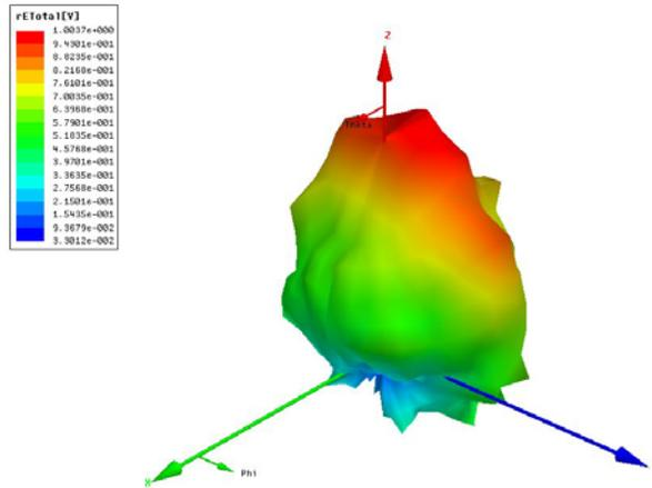
Figure 2. 3D plot of the radiated far field intensity of the cow mounted collar antenna in-situ with the cow in the nominal pose. The axis is the same as for Fig. 1(a) with the cow's head pointing in the positive x-direction. Most of the radiation is directed upwards.
