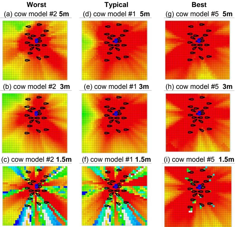
Figure 7 Horizontal signal coverage (plan view) for receivers located at a height of 1.5m – 5m in a pasture with a small herd of cows: (a-c) worst case, (d-f) typical case, (g-i) best case, Red squares indicates the strongest signals (-70dBm), green the midstrength (-86 dBm) and blue the weakest (-110dBm). Each square represents an area of one metre.
