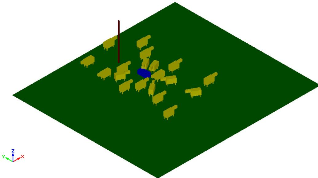
Figure 6. Rendering of the simulation setup in RPS for modelling a pasture with a small herd of 20 cows. The pasture is 36m long and 36m wide. The telephone pole is 8m high. The cows are shown in yellow. A plastic water trough, filled with water, is shown in blue.
