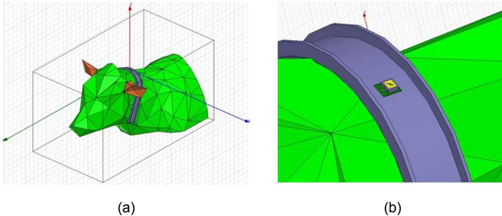
Figure 1. 3D rendering of optimised cow, collar and antenna model mesh for electromagnetic simulation purposes: (a) the head neck and shoulders cow model are sufficient for accurate modelling (b) detailed view of the patch antenna located at the top of a metal collar with flanges.
